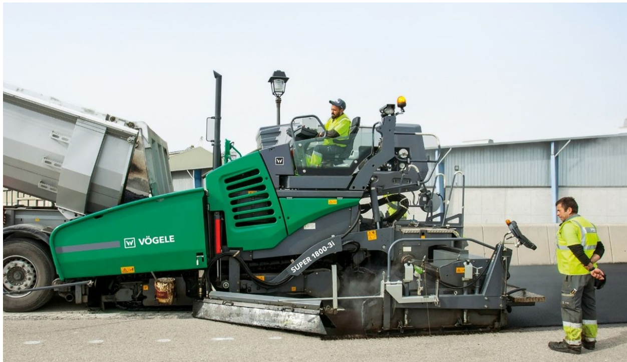
Figure 13.24-3b. Typical Spray Paver
